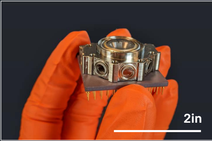
IonQ ion trap and vacuum chamber in a single, minuscule package 1
