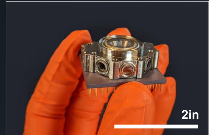
IonQ ion trap and vacuum chamber in a single, minuscule package
