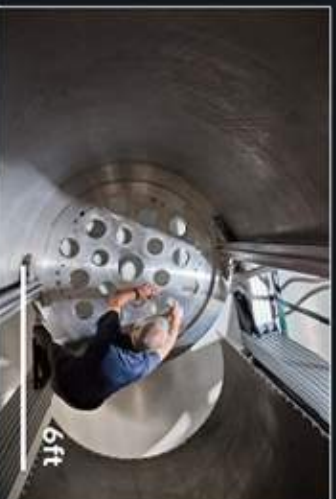
An IBM engineer working on the custom-built dilution refrigerator casing for a single QPU
