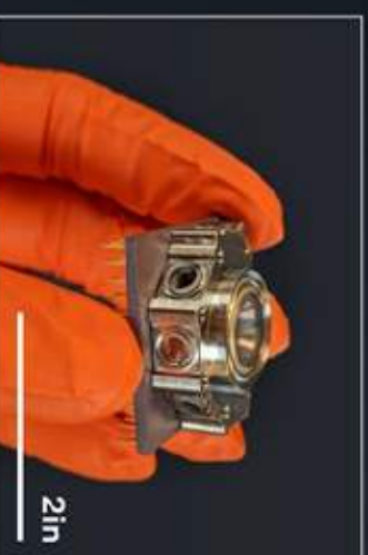
IonQ ion trap and vacuum chamber in a single, minuscule package 1
